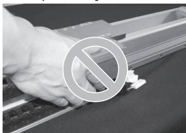
Do not transport the actuator by holding its slider.
