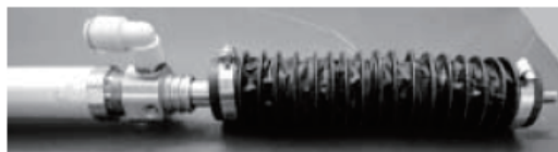
Removal of bellows
