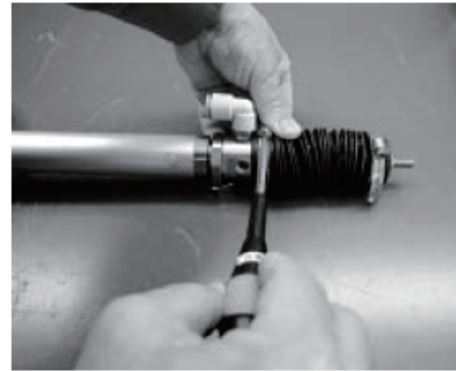
Loosening of rear metal fitting
