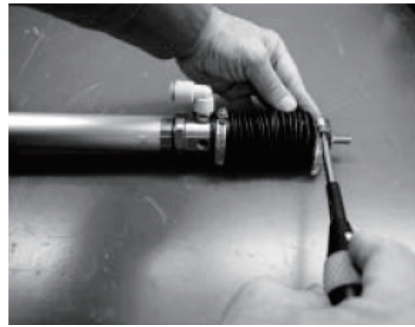
Tightening of front metal fitting
