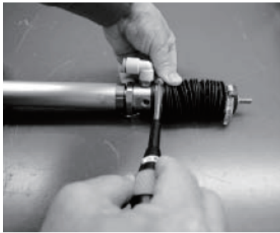
Tightening of rear metal fitting
